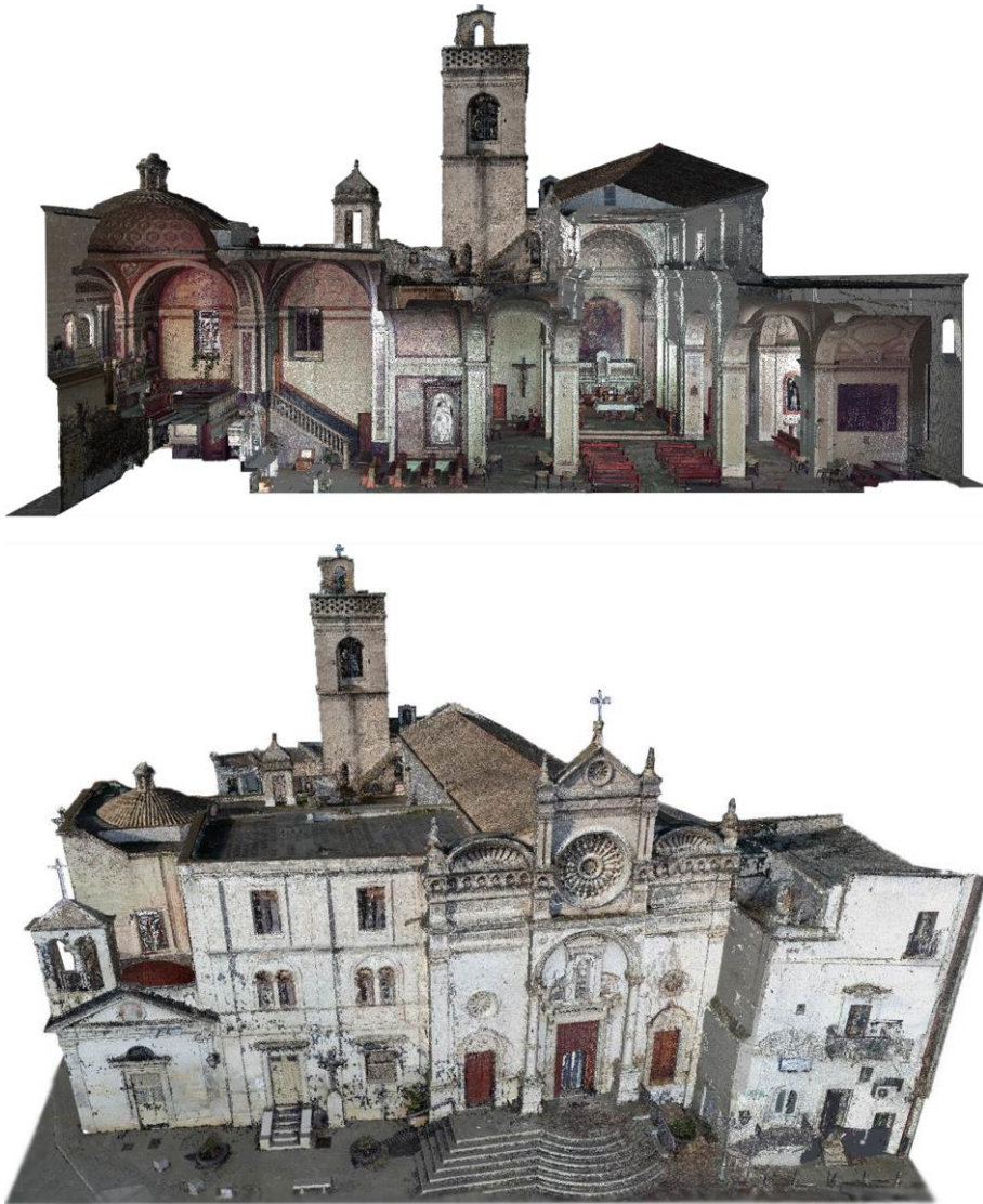
Fig. 22 Integrated point cloud: internal view (on the top) and external view (on the bottom).
