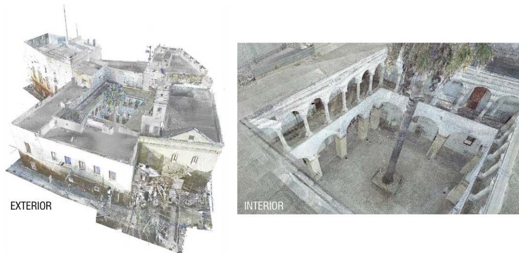
Fig. 34 Point cloud: external view of the entire complex (on the left); internal view of the courtyard (on the right).
