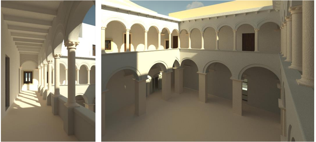
Fig. 38 3D model rendering of the portico on the second floor (on the left) and the inner cloister (on the right).
