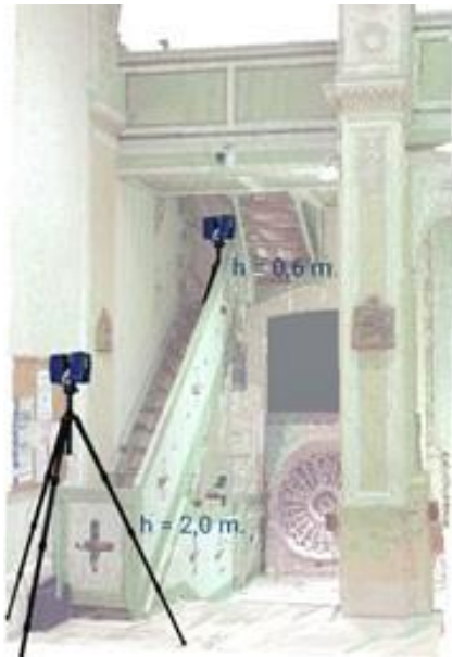
Fig. 17 Laser scanner stationing at different instrumental heights.
