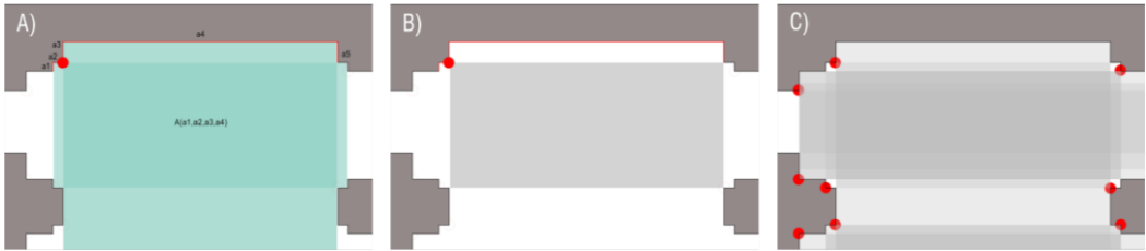
Fig. 108 A) Overlapping of the five visibility areas; B) Common visibility area for the selected vertex; C) Overlapping of calculated visibility areas for the vertices within a section of the church’s interior.
