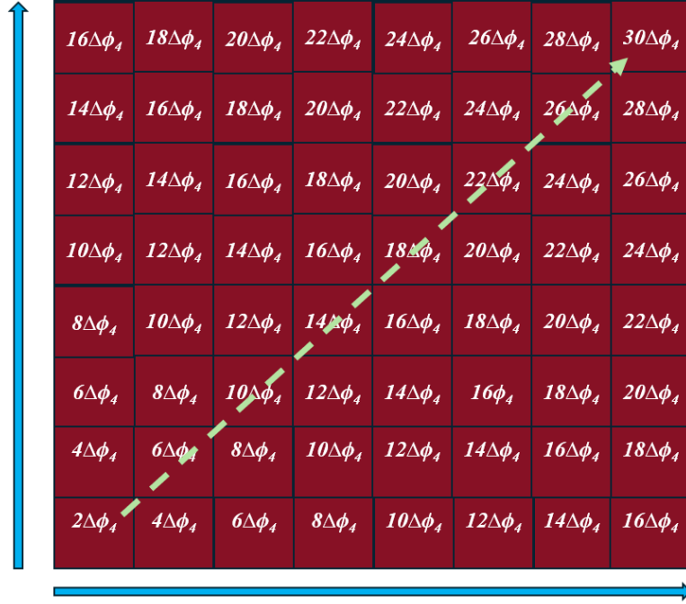
Fig.3.5 Schematic of phase gradients in horizontal and vertical direction.
