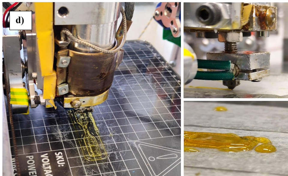
Fig.B5-: d) printing of the dogbone specimen (DCT = On, Text = 145°C).
