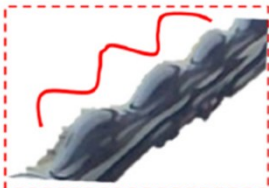
Fig. 3.6: Electromagnetic assistance to improve the printing quality, tested on the proposed soft ink (Ecoflex 00–10 +30 wt% of \text{Fe}_3\text{O}_4 ). a) Effect of different current inputs (0 A, 3.5 A, and 4.5 A) provided to the copper coils to generate electromagnetic force on the printing quality, and b) benefits of the proposed approach in overcoming over-extrusion problems when a layer height of 0.1 mm is set.
