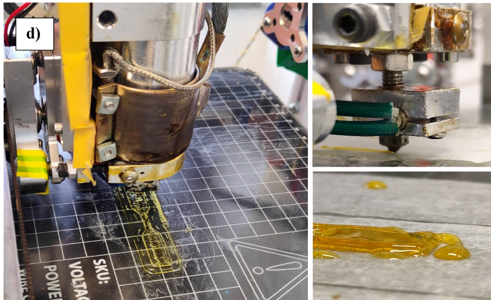
Fig.B5-: d) printing of the dogbone specimen (DTC = On, Text = 145°C).
