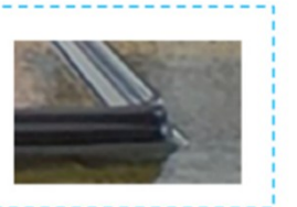
Fig. 3.6: Electromagnetic assistance to improve the printing quality, tested on the proposed soft ink (Ecoflex 00–10 +30 wt% of \text{Fe}_3\text{O}_4 ). a) Effect of different current inputs (0 A, 3.5 A, and 4.5 A) provided to the copper coils to generate electromagnetic force on the printing quality, and b) benefits of the proposed approach in overcoming over-extrusion problems when a layer height of 0.1 mm is set.
