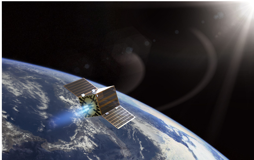
Figure 4: Render of the Multi-Application Minisatellite with a recurrent platform, compatible for multiple launchers and missions
