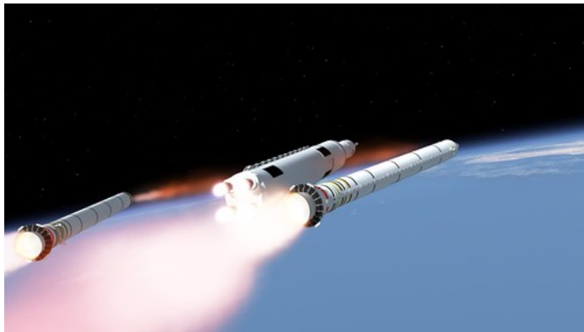
Figure 2: Space launch system booster separation that causes shock loads
