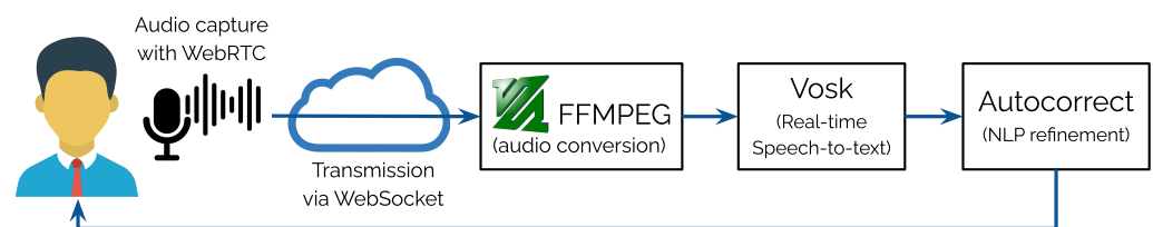
Figure 1. Overview of the system architecture, showing the interaction between the client interface, WebSocket communication channel, server-side processing modules (audio conversion, STT, NLP), and the final display of the transcribed text.
