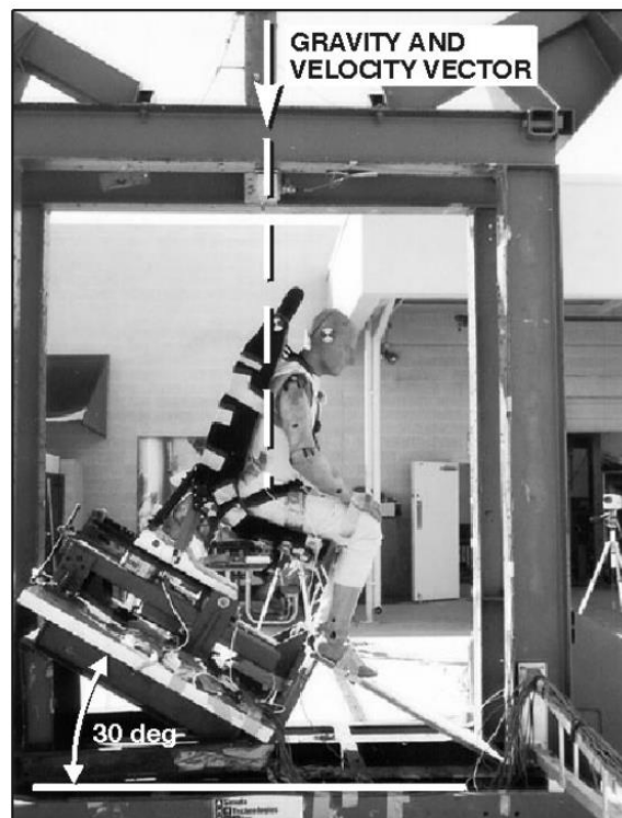
Figure 23 Dynamic Impact Test 1: As conducted on a drop tower with the seat tilted 30-deg nose-down [12].
