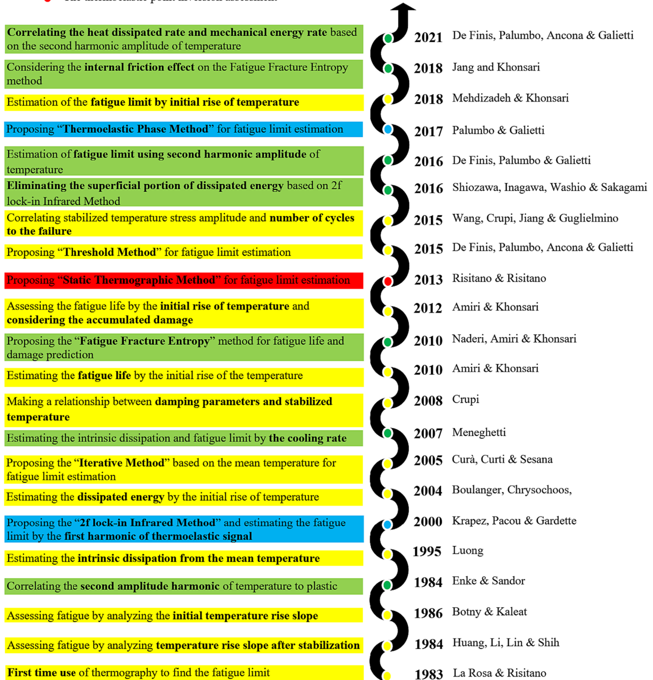
FIGURE 1 Some milestones in developing the history of thermographic techniques for fatigue assessment. [Colour figure can be viewed at wileyonlinelibrary.com ]
