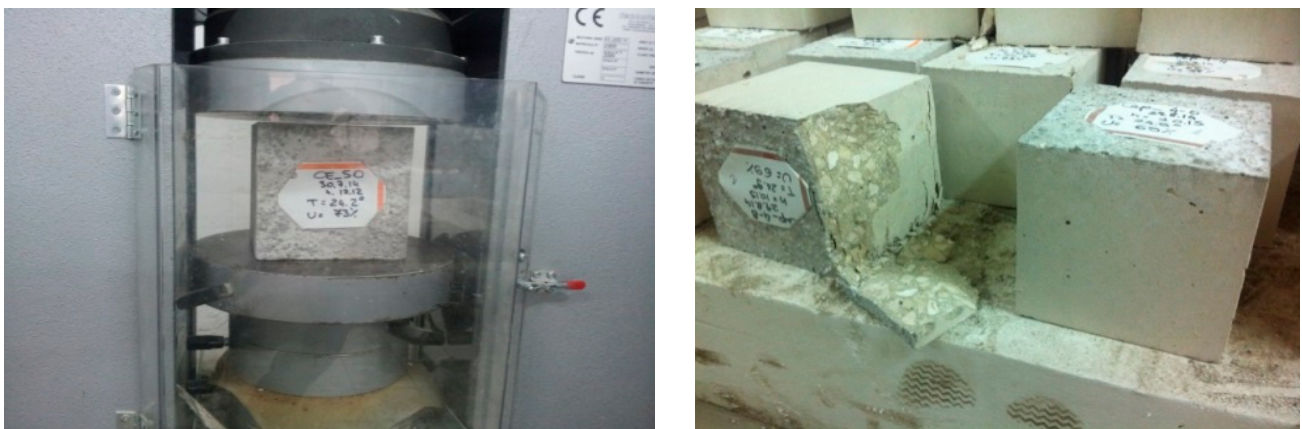
Figure 7. Compression test on concrete specimens.
