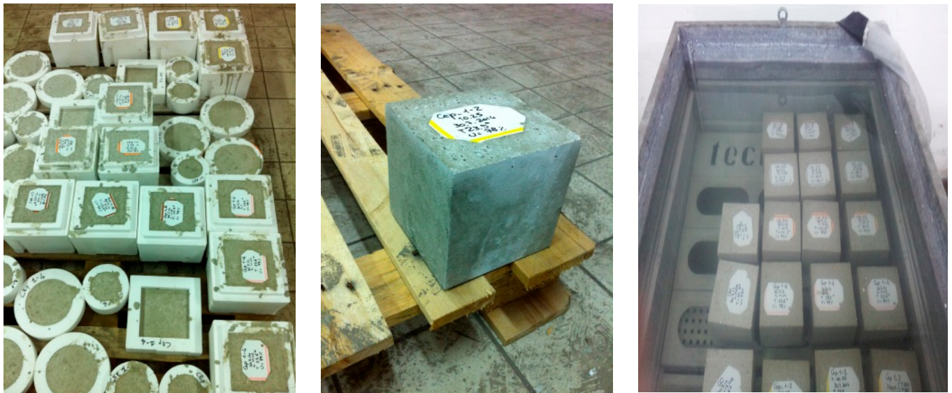
Figure 6. Preparation of concrete specimens, demolding, and conditioning in a tank.
