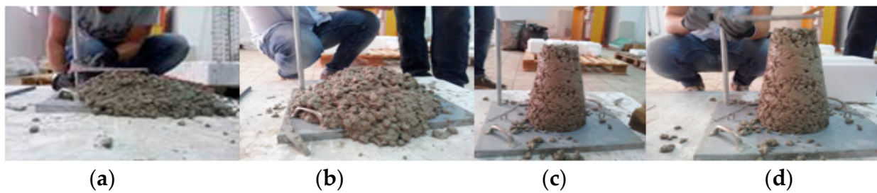
Figure 17. Concrete. Flow test S4 (a,b) and S6 (c,d).
