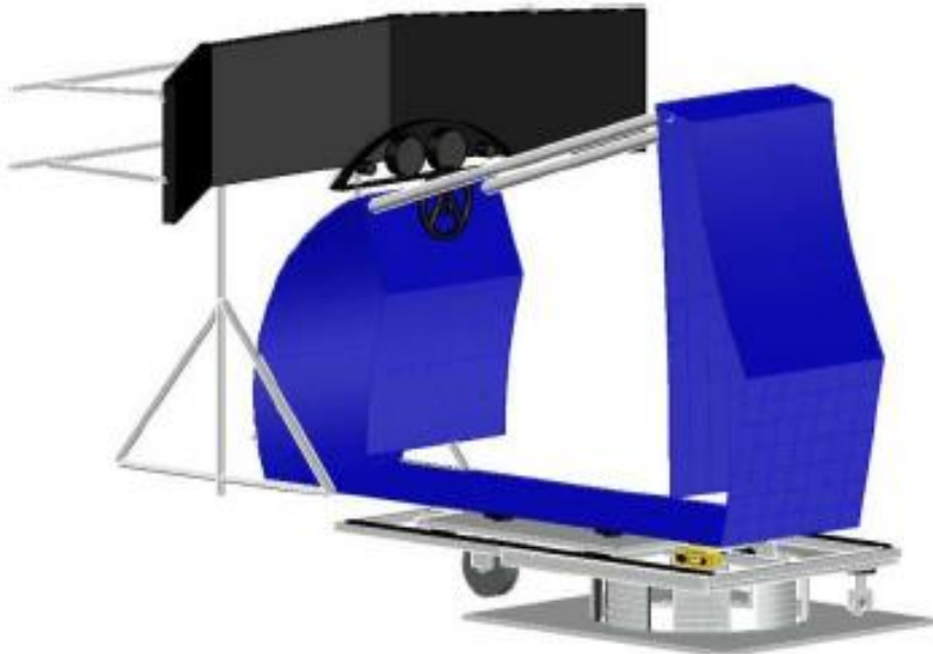
Figure 9 – Simulator cabin and motion cueing platform - Driving simulator PICS-L, Université Gustave Eiffel
