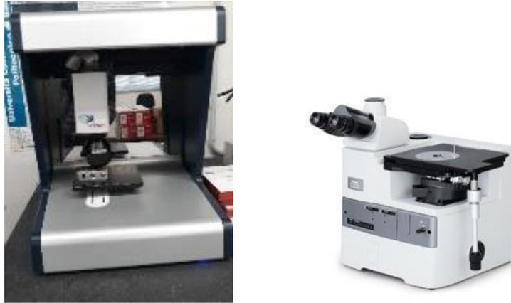
**Figure 3-15.** Left: High Precision Conoscan; Right: Nikon Eclipse MA200 microscope.
