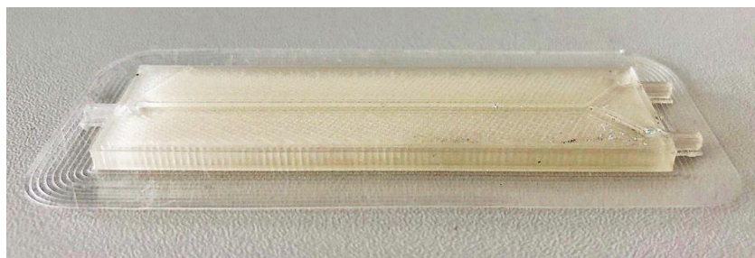
Figure 3-9. FFF 3D-printed micromixer with brim after removing from the build plate.
