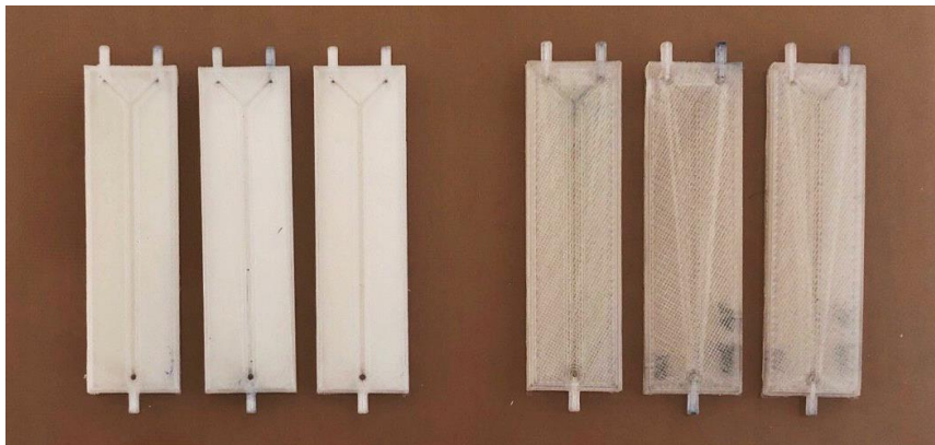
Figure 4-19. Two printed channels. Left: channel 1 with a line width of 200 \mu\text{m} ; Right: channel 2 with a line width of 600 \mu\text{m} .
