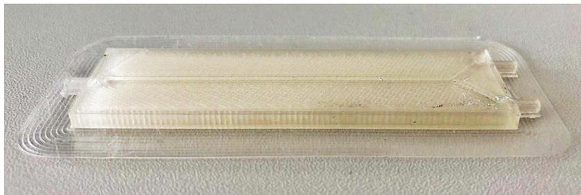
**Figure 3-9.** FFF 3D-printed micromixer with brim after removing from the build plate.
