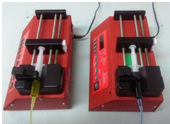
Figure 3-18. BS-300 Braintree syringe pumps for injecting solutions with disposable syringes.
