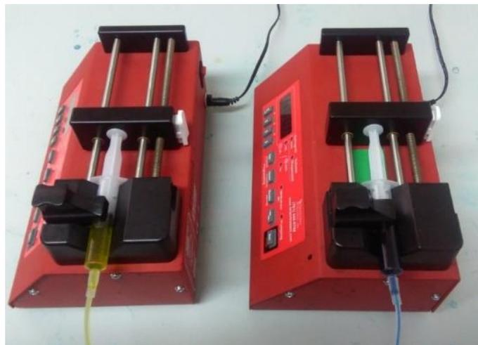
**Figure 3-18.** BS-300 Braintree syringe pumps for injecting solutions with disposable syringes.
