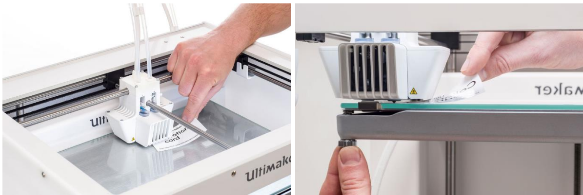
Figure 3-8. Manual calibration of the Ultimaker printers using calibration card.
