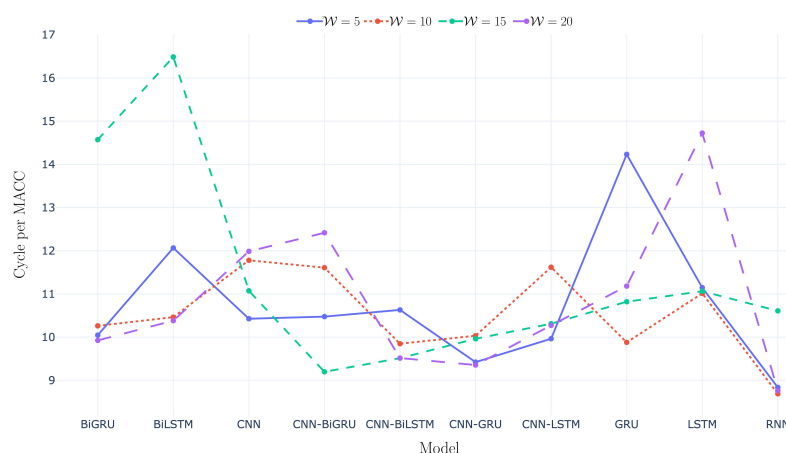
Figure 4.10: Comparison, in terms of number of cycles per MACC, between the considered ML and DL models for different values of the time lag \mathcal{W} .
