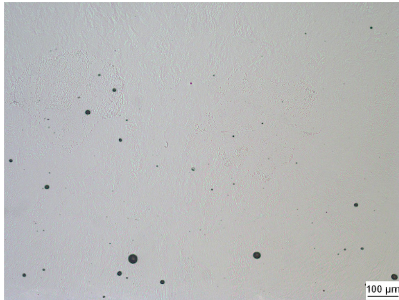
Figure 72 - Optical micrograph of 5_C specimen showing porosity.
