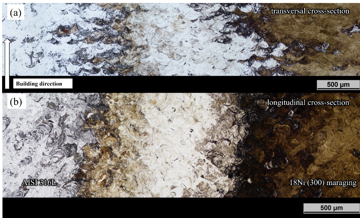
Figure 18 - Optical micrograph of the test specimen (Batch 2) interface for metallographic analyses at 100 magnification: (a) cross-section showing the building direction; (b) longitudinal section showing the single layer. The phase information can also be detected by the matching hardness values, where austenite exhibits a hardness lower than 300 HV whereas martensite can be as hard as 600 HV (see
