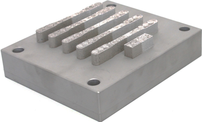
Figure 17 - Image of specimens made for tensile tests and metallographic examinations.
