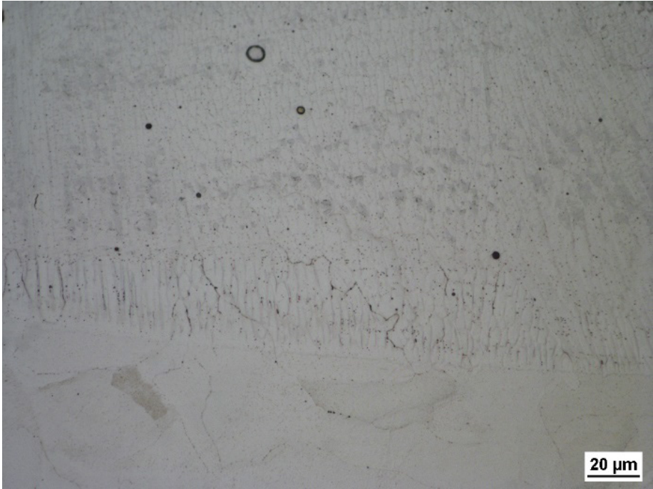
Figure 75 - 1_T specimen microstructure showing the incomplete martensitic transformation.
