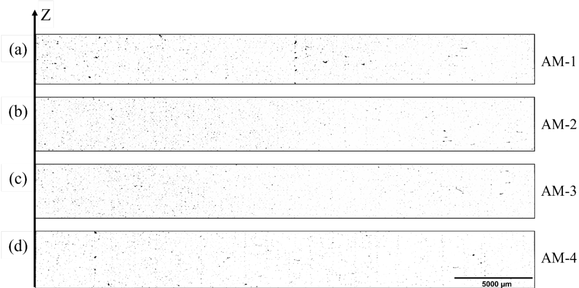
Figure 50 - Appearance of the metallographic specimens after threshold application.
