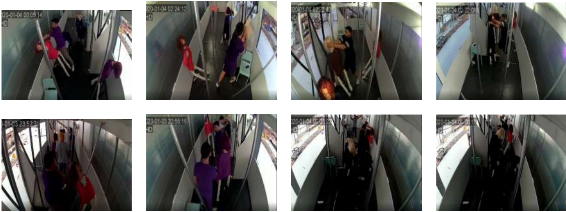
Figure 3.8: Representative examples of low-occupancy scenes (top row, fewer than four individuals) and high-occupancy scenes (bottom row, at least four individuals) for both Fight and No Fight classes in the laboratory dataset. All scenes were recorded in a controlled experimental environment using human-sized mannequins to systematically reproduce varying passenger density conditions.
