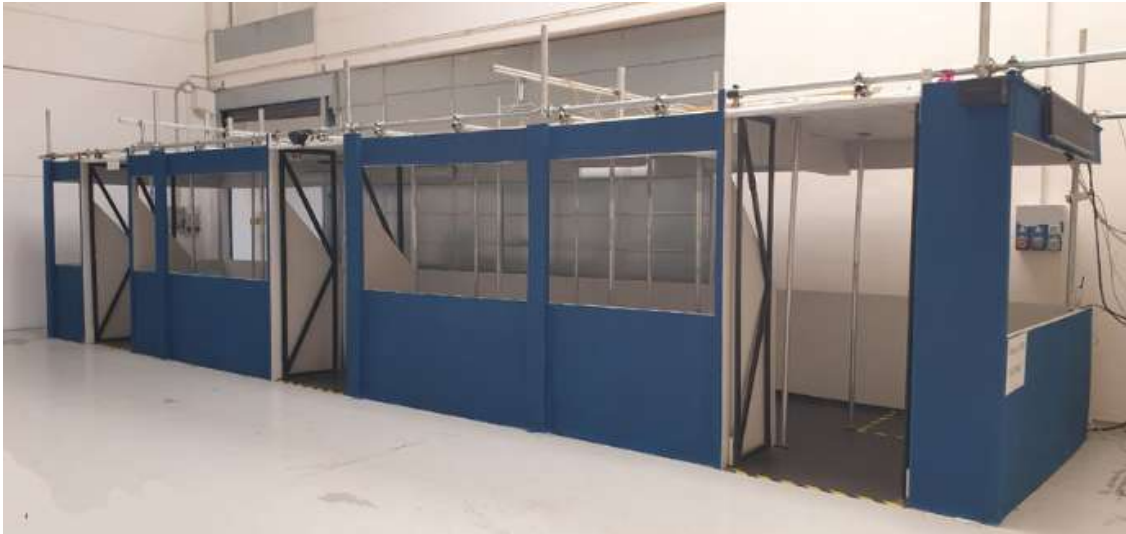
Figure 2.2: Laboratory simulator (full-scale 1:1) reproducing the target bus interior (aisle, seats, poles, doors).
