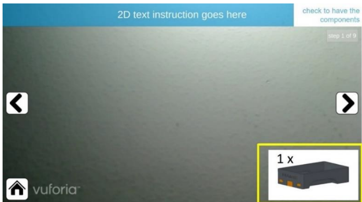
Fig. 6 Example of displaying the information type IDENTITY through a drawing (highlighted in yellow) screen-fixed, static, with the colors of the real truck bed.
