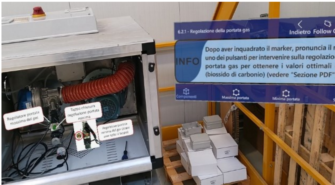
Fig. 20 Example of an "AR scene" of the developed MRTD about gas flow adjustment.
