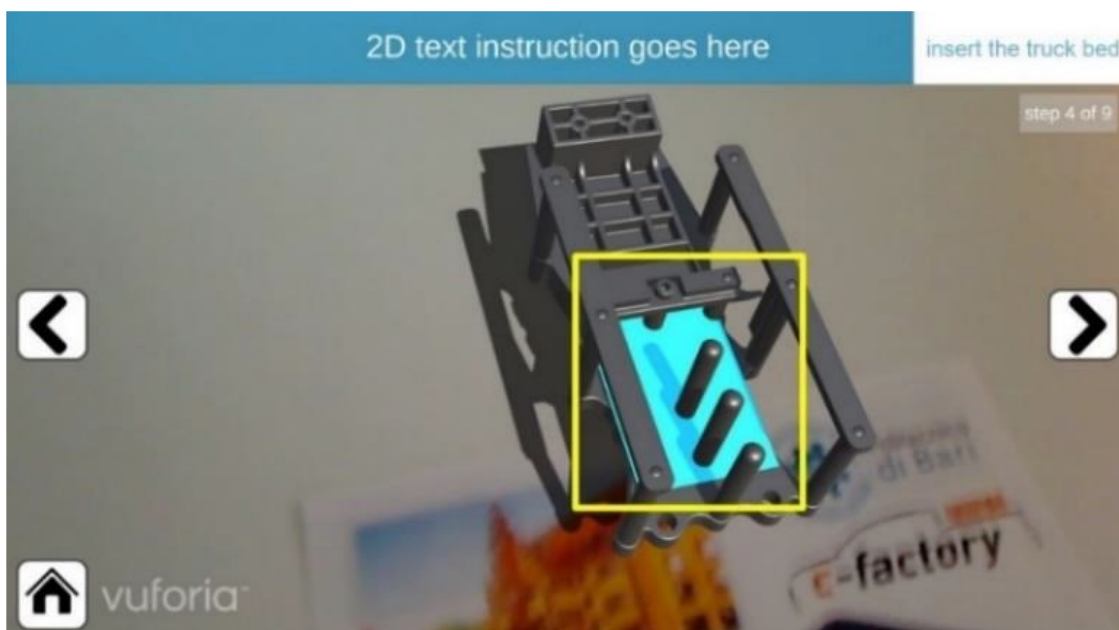
Fig. 7 Example of displaying the information type LOCATION through an AM (highlighted in yellow) world-fixed, without color coding and static.
