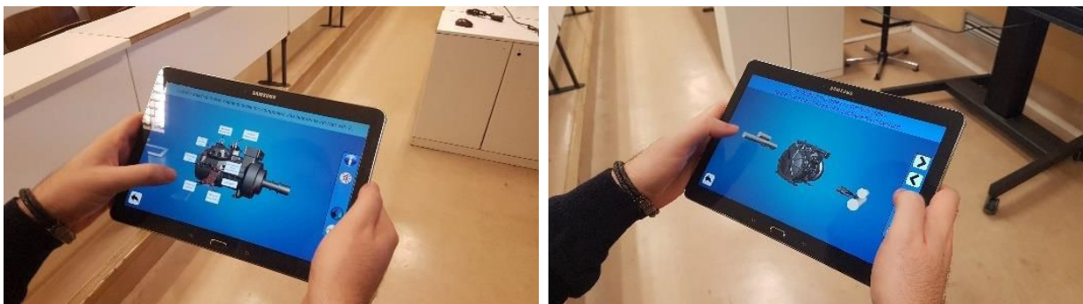
Fig. 46 User interaction example of the DVR demo version: the handheld device shows the 3D model of the compressor and the AR content, consisting of the proposed visual assets, in an entirely virtual environment.
