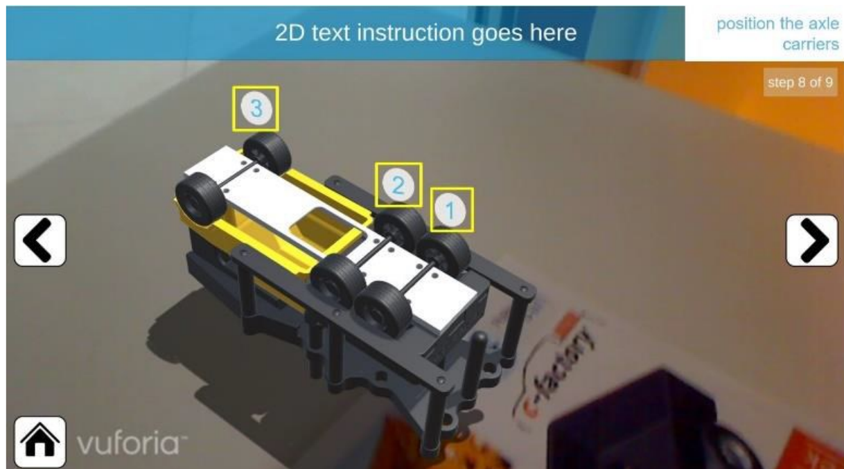
Fig. 10 Example of displaying the information type ORDER through an animated world-fixed text (highlighted in yellow) without a color coding.
