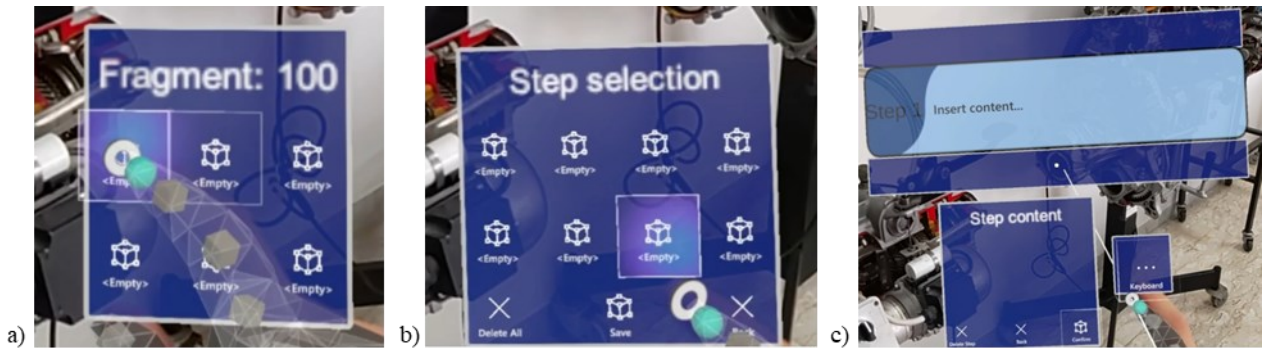
Fig. 42 SMARTDOC hand menu with the save slots of each operations sequence (a), the step selection (b), and the textual instruction insertion (c).
