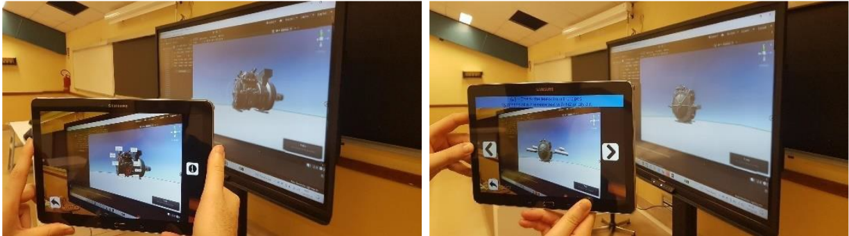
Fig. 47 User interaction example of the ADVR demo version: the handheld device shows the AR content, consisting of the proposed visual assets, referenced to the 3D CAD model of the compressor displayed on a secondary screen.
