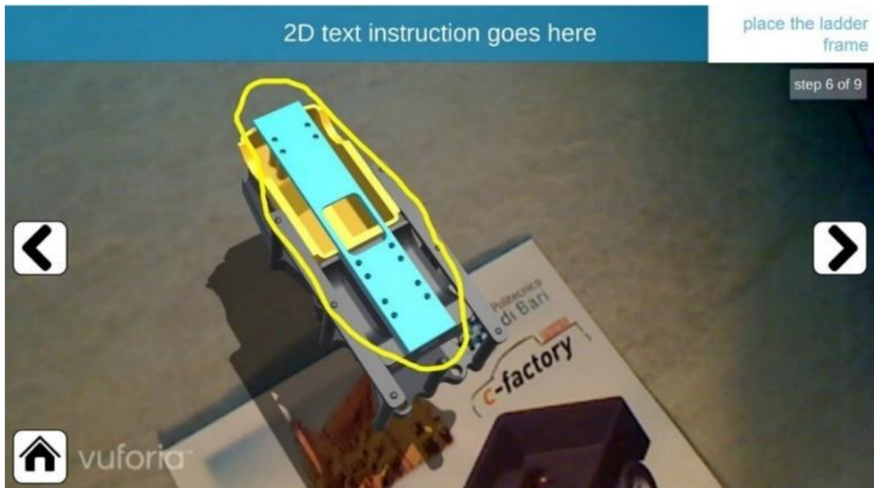
Fig. 11 Example of displaying the information type ORIENTATION through a static world-fixed product model (highlighted in yellow) without a color coding.
