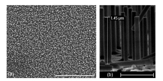
**Figure 3.** SEM images of Al/Si nanopillars obtained with our fabrication technique: (**a**) on a large zone (scale bar =  $20 \ \mu$ m); and (**b**) cross-section view of the nanopillars (scale bar =  $1 \ \mu$ m).
