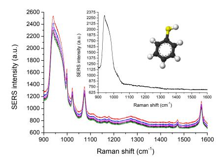
**Figure 4.** Five SERS spectra of thiophenol molecules recorded randomly on the whole substrate composed of Al/Si nanopillars. The inset depicts the Raman spectrum of thiophenol obtained with only Si nanopillars (without metal). Moreover, the molecular scheme of the thiophenol molecule is also displayed.
