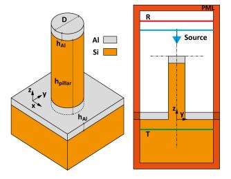
**Figure 2.** Nanopillar morphology used for the FDTD simulations, the diameter (*D*) is 150 nm, the height  $(h_{pillar})$  is 1450 nm, and the Al layer thickness  $(h_{Al})$  is 50 nm on the top of nanopillar and on Si substrate. On the right, the broadband plane wave source and monitors (R and T) for calculating the extinction spectrum are displayed.
