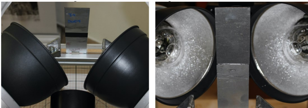
Figure 79. Experimental set-up in reflection configuration. (a) The front surface of specimen with black coating. (b) The back surface of specimen with embossing.
