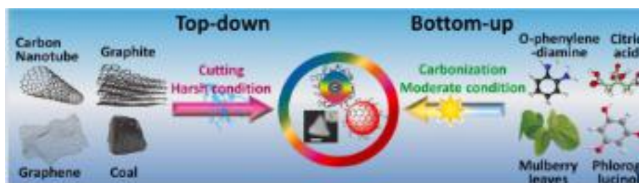
Figure 1.2: Schematic illustration of division between top-down and bottom-up synthetic techniques for CDs. Adapted from [65].
