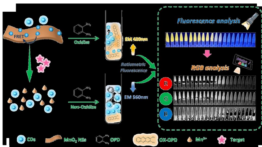
Figure 1.11: Schematic description of the working principle of a ratiometric fluorescence-based colorimetric sensor for the portable detection of antioxidants with smartphone detection, reproduced from [183].
