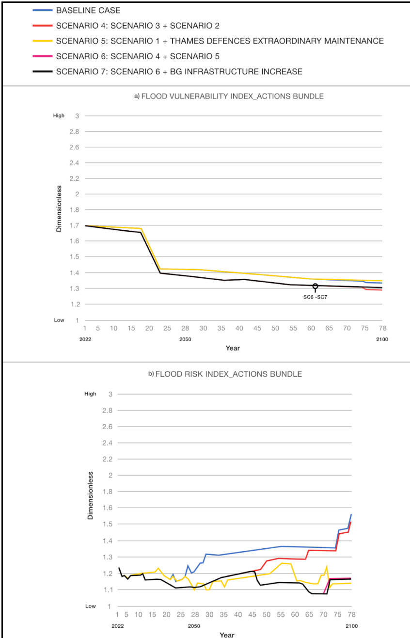
Fig. 31 – a) ‘flood vulnerability index’ and b) ‘flood risk index’ outputs of Scenarios 4–7 using the baseline case as reference. Where scenarios overlap, their labels are placed and separated by a hyphen (-).
