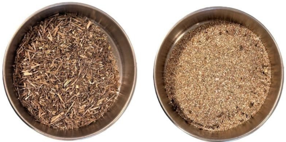
Figure 14- Mix 1 Posidonia oceanica 2 mm < D < 5 mm, Sand D < 1 mm
