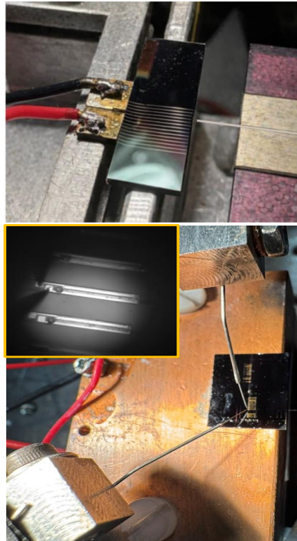
Fig. O3: Fiber-free HECL based on butt-coupling between gain chip and SiN PIC. (top) Two-chips HECL, (bottom) transfer printed HECL.
