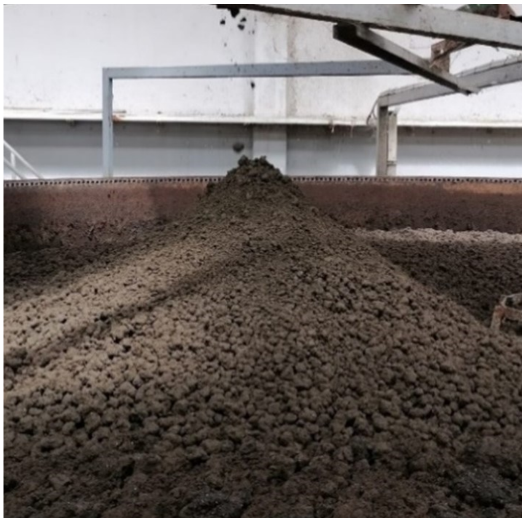
Figure S12. Stabilized sludge.
