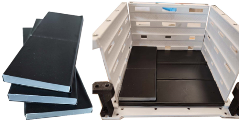
Figure 2.6: Photo of the realization of the structural model of the PST. In the flight model Aluminum foil will replace black vinyl tape.
