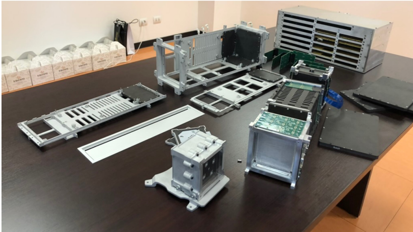
Figure 6.7: Ziré structural model for vibration tests.
