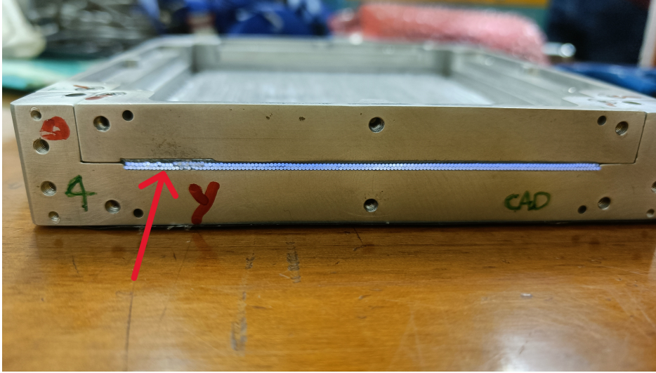
Figure 6.24: Photo of one side of the Y-view plane of the FTK module with the glue on the whole fiber length. The red arrow indicates the defect in the fiber positioning.
