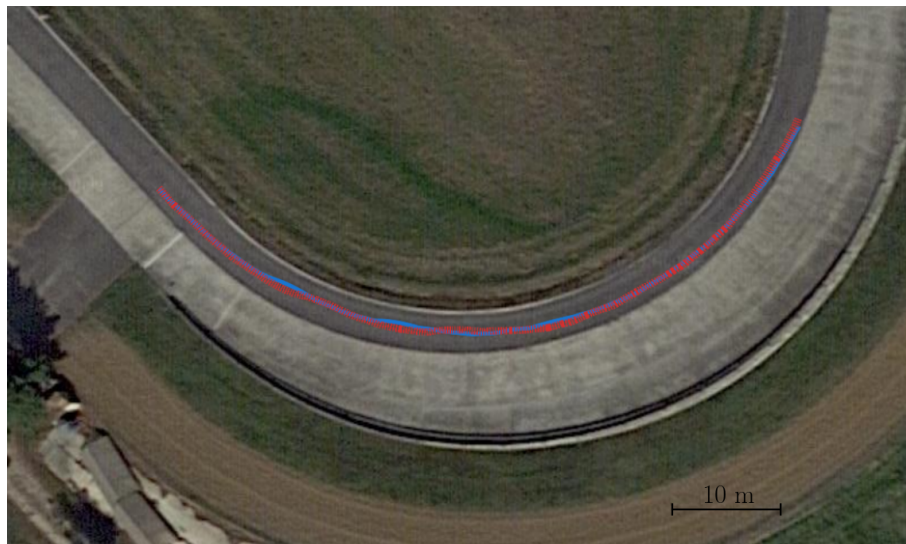
Figure 4.30: Comparison between measured (dashed red line) and simulated path (solid blue line) followed by the robot during the validation test on a curved path. GPS coordinates of the test site (DMS format): 44^{\circ} 57' 24.5988'' N, 7^{\circ} 33' 25.956'' E).
