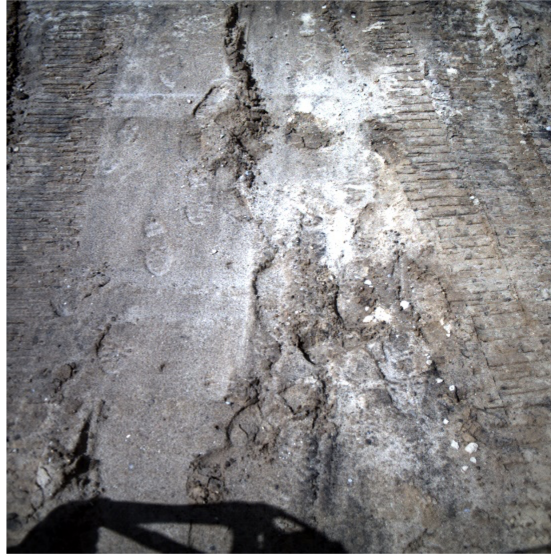
Figure 4.4: Close up of the tracks left by the wheels of SherpaTT during the sand mine testing.
