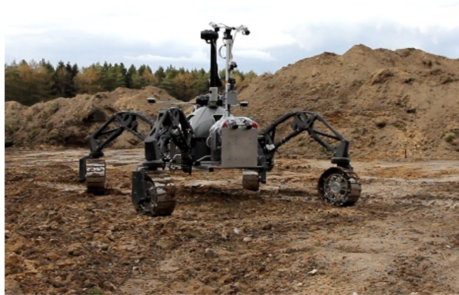
Figure 4.3: Sherpa TT during the sand mine testing.
