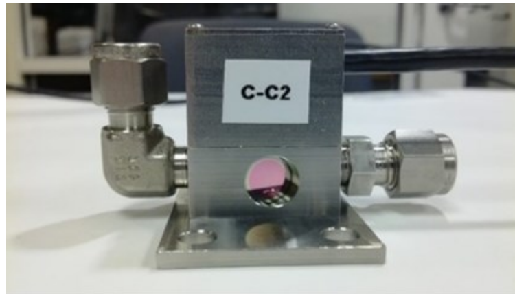
Figure 1.2 Photograph of an ADM. An optical window and the gas inlet and outlet connectors are also visible.
