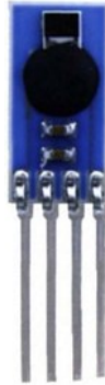
Figure 4.11 HYT271 sensor. Pinout (from left to right): SDA (serial data), GND (ground), VDD (positive power supply), SCL (serial clock).
