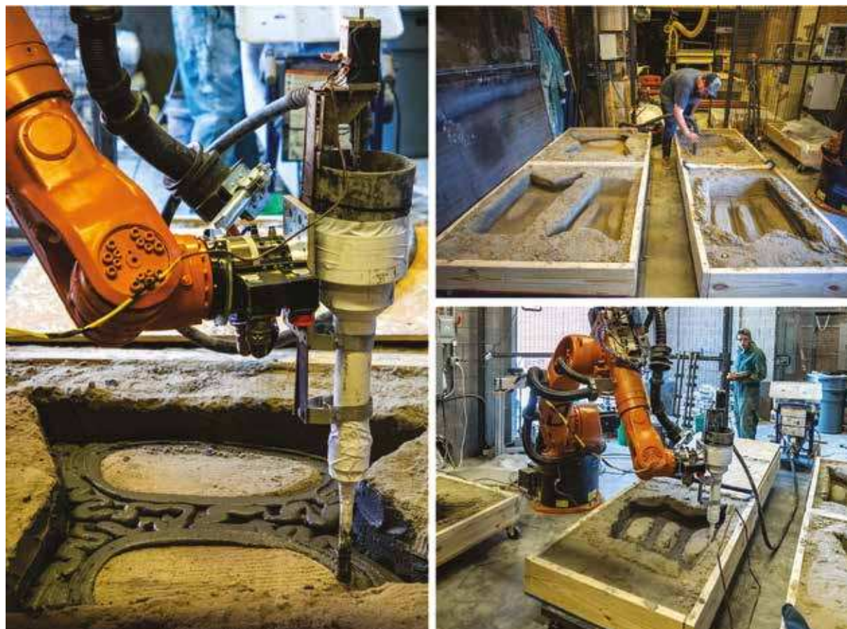
Figg. 70-72. Il Sub-Additive Concrete Printing Method (© Christopher Battaglia, Martin Miller, Kho Verian).
