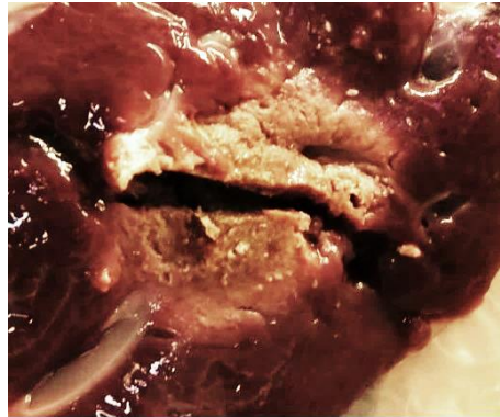
Figure 3.27 Thermal lesion in bovine liver obtained during the experimental ex-vivo validation produced using a power supply of P_{avg} = 10 W for t = 180 s . 14G MW applicator prototype [2].
