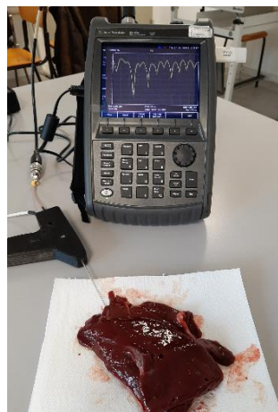
Figure 3.28 Experimental measurement of the scattering parameter modulus |S_{11}| of 16G MW applicator prototype [4].
