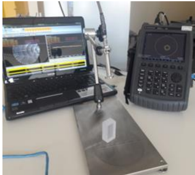
Figure 3.15 Set-up for the dielectric characterization of a biocompatible 3D printing material for the insulating section and measured sample
