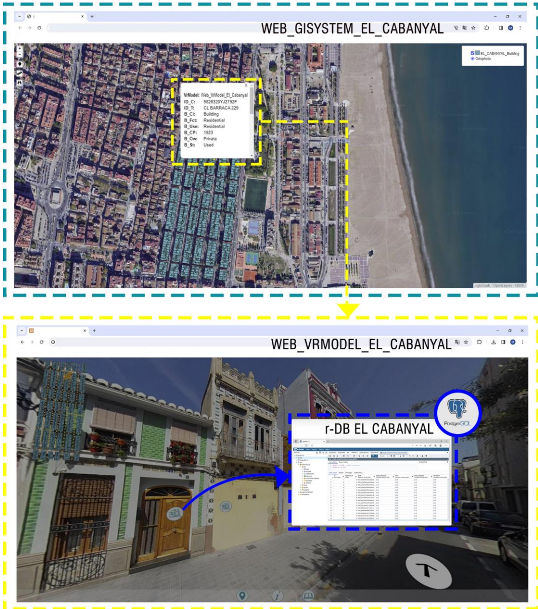
Figure 50 - Home screen of the Web-GiSystem showing the query of an architectural entity. The information window allows the connection to the Web-VrModel, as well as the implementation of further data, remotely on-desk, in the r-DB.
