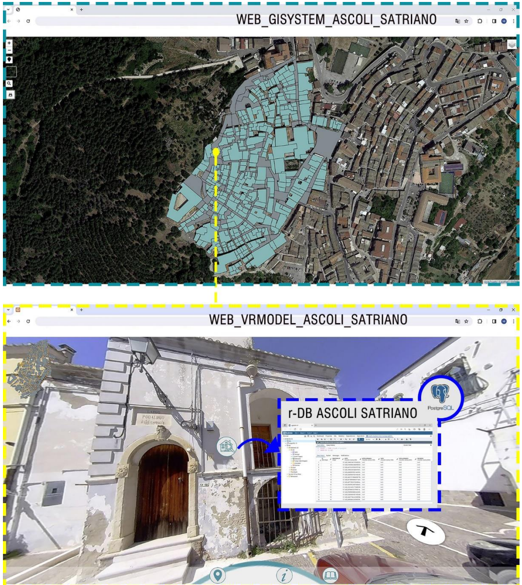
Figure 59 - Home screen of the Web-GiSystem showing the query of an architectural entity and the link to the Web-VrModel. The Web-VrModel screen shows the implementation of additional data in the r-DB remotely on-desk
