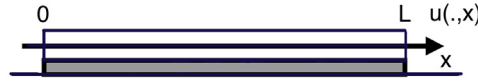
Fig. 1. Thermoelastic one-dimensional body interacting through an adhesive layer (in gray) with a rigid substrate.
