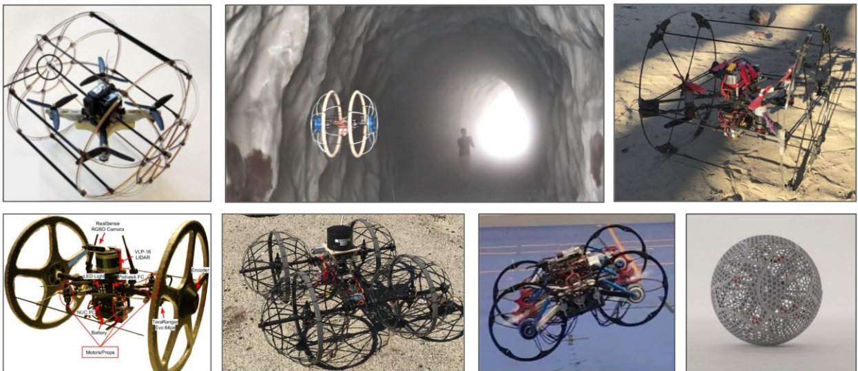
Figure 6-50: Hybrid platform hardware evolution (top row: left to right) pre-challenge Hytaq design [103], Modular hybrid vehicle [105], (bottom row: left to right) Autonomous Rollocopter [102, 29], DrivoCopter [107], BAXTER [108], Spherical Rollocopter [109, 110].
