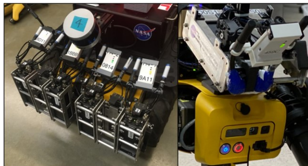
Figure 6-44: NCDS equipped on Husky (left) and Spot (right).
