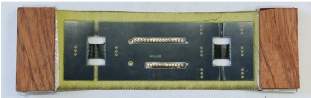
Figure 2-6 FRET specimen ready for the Tensile test
