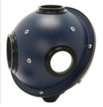
Figure 24: Picture of the integrating sphere, showing the entry port ( 90^\circ ) and the two exit ports, P1 ( 0^\circ ) and P2 (North pole), all oriented perpendicular to each other.
