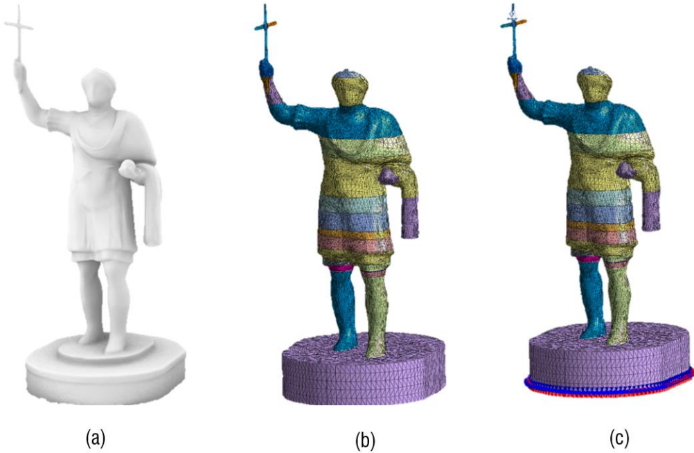
Fig. 6.11 - Parametric 3D model for FEM analysis: NURBS processed in Rhino software (a), structural mesh (b), base constraint condition (c).
