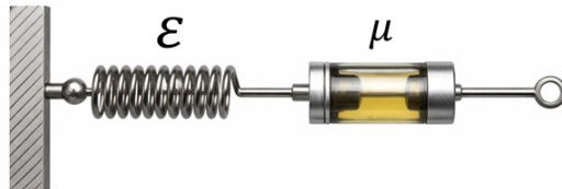
Figure 1.6: Schematic representation of the Maxwell viscoelastic model.
