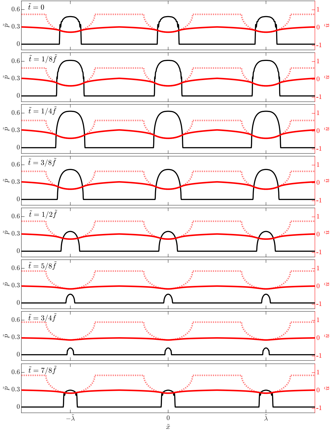
Figure 2.7: The pressure distribution at different time steps is characterized by the black line and the corresponding displacement distribution, the red line. The dotted red line shows the change in the position of the rigid indenter. In the simulation, the average displacement value is \tilde{\Delta}_0 = 0.25 , the oscillation frequency is \tilde{\alpha} = 3.12 \times 10^{-10} and the amplitude is \tilde{\alpha} = 0.15 .
