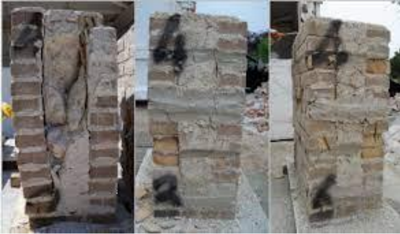
Fig. 3. 5 – Multi-leaf masonry wall.
