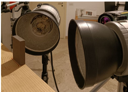
Fig. 7 Experimental setup adopted for pulsed thermographic tests: energy source with two flash lamps and MWIR cooled sensor FLIR A6751
