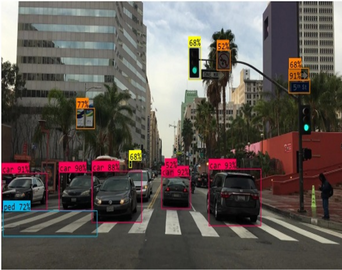
Figure 2.33: Detected objects from front and rear image of car dataset with complex background—the first test dataset.
