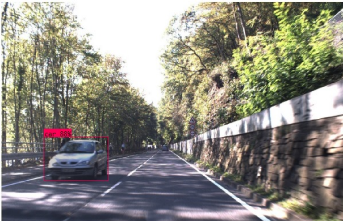
Figure 2.32: Detected car in suburbs from traffic signs dataset in YOLO format.
