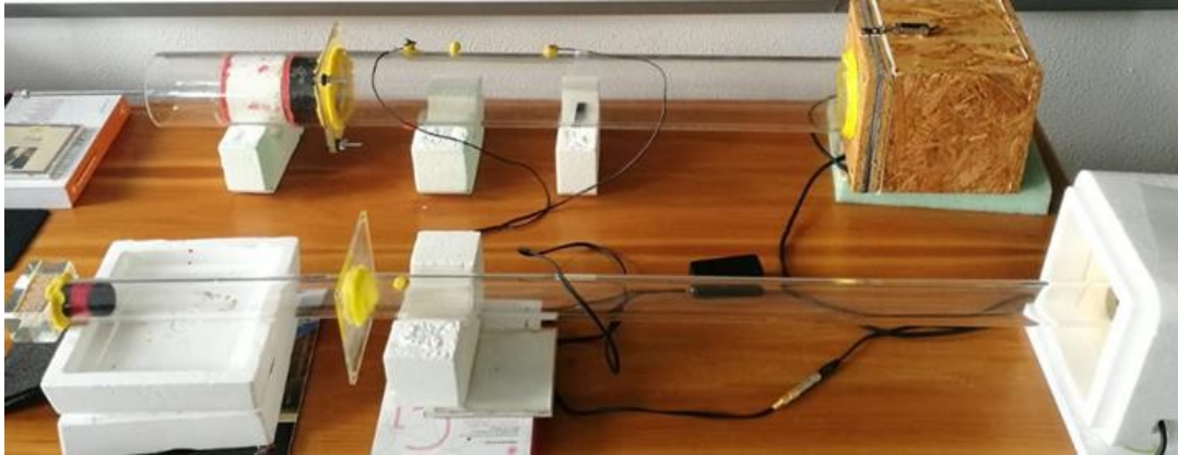
Figure 3.3. Standing wave tubes used for sound absorption at low and medium frequencies (top), and at high frequencies (bottom).
