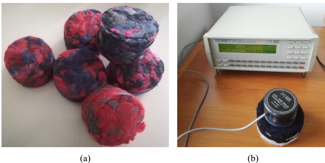
Figure 3.1. Samples (a) and apparatus for testing thermal properties (b).
