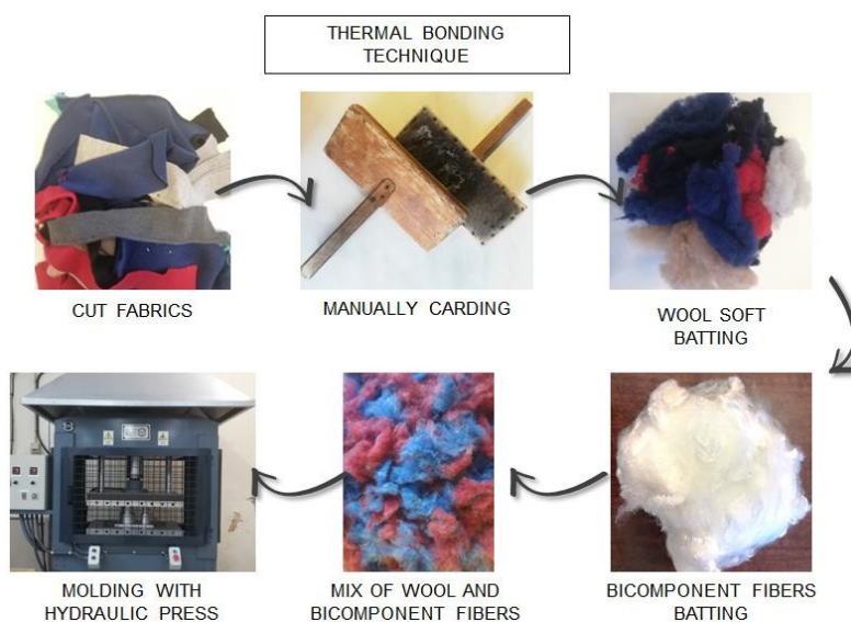
Figure 2.10. Main steps of the thermal bonding process.
