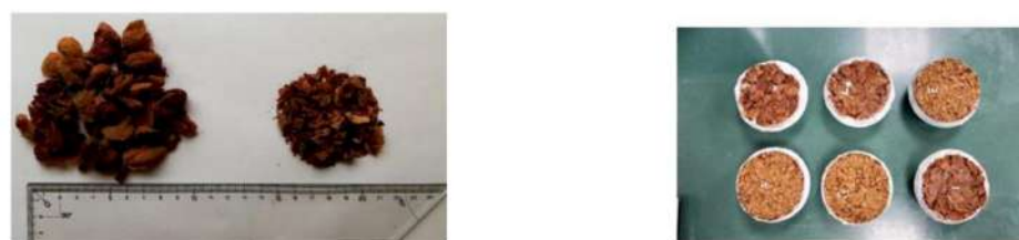
Figure 3. Sound absorbers made with almond skin waste (Liuzzi et al. [30]).
