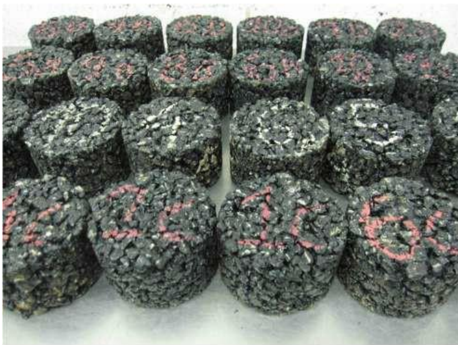
Fig. 2. Some samples after the ITS test.
