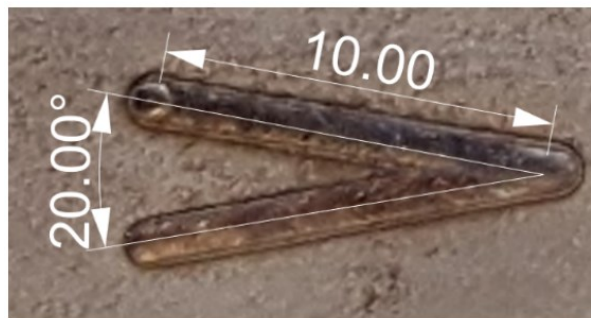
Figure 45. V-track depositions tests [82].
