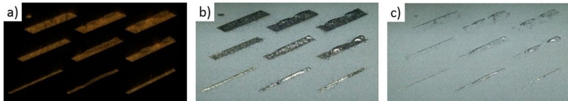
Figure 87. Layer 800 of sample S3-T3 signaled as out of control. (a) OT of the whole layer, (b) scanned layer image, and (c) powder bed recoating [72].
