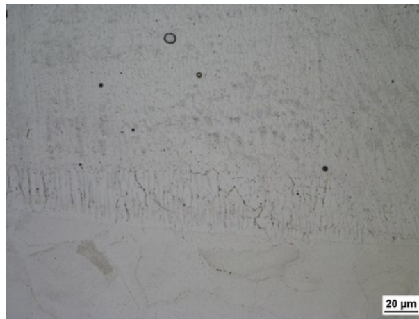
Figure 152. 1_T specimen microstructure showing the incomplete martensitic transformation [155].
