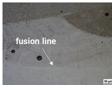
Figure 151. Optical micrograph of the interface zone in specimen 5_T at 200X magnification [155].
