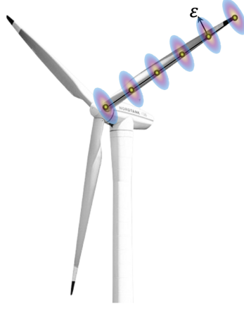
Figure 2.5: Scheme of the Actuator Line Model, where the Gaussian kernel \eta distributes the aerodynamic forces around the actuator lines.
