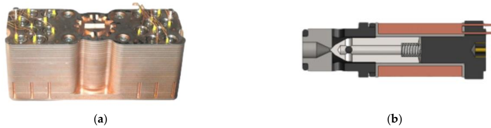
Fig. 61. DFCU with sixteen on/off valves in parallel developed by Paloniitty et al. [210]: (a) prototype; (b) utilized on/off valve.
