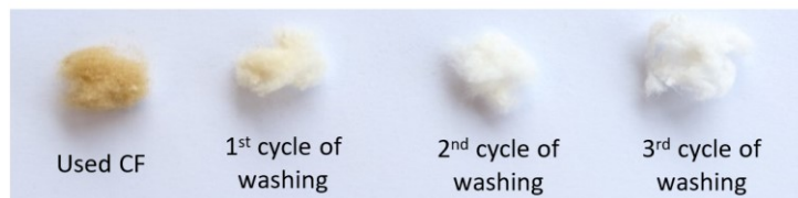
Figure 3.18 Cellulose acetate fiber after purification in 75% ethanol multiple cycles
