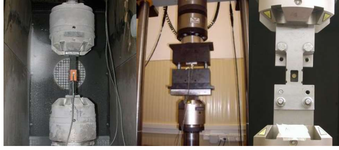
Figure 1. Set up for tensile, compression and compression filled hole tests.
