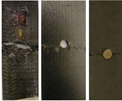
Figure6. Typical fracture for compression, compression open hole and filled hole.
