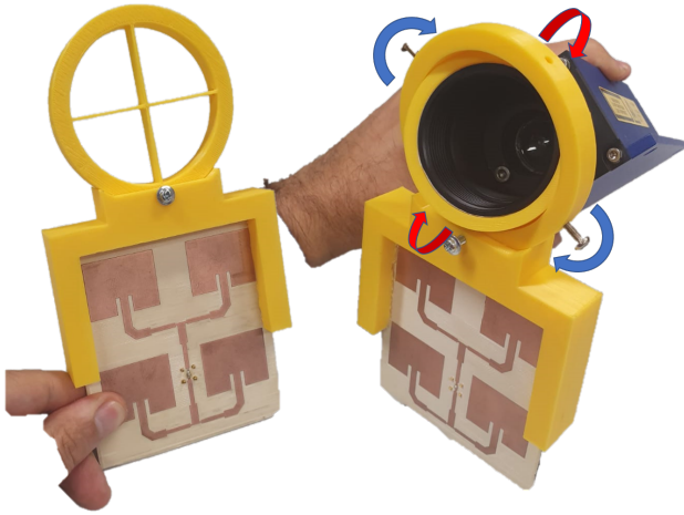
Fig. 15: Laser pointing structure
