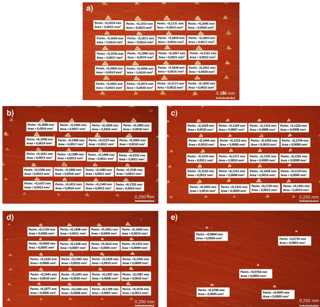
Figure 4.3. Optical micrographs of cross-sections: (a) untreated, (b) 50 % EA – 7 min, (c) 50 % EA – 10 min, (d) 75 % EA – 7 min, (e) 75 % EA – 10 min. Progressive reduction in interlayer voids with increasing treatment intensity is evident (Iqbal et al., 2024).
