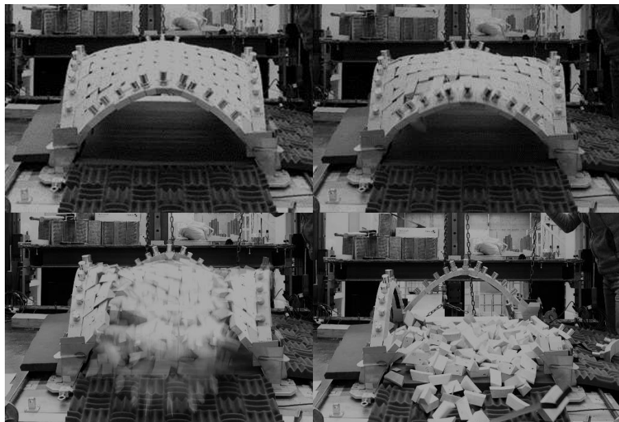
Figure 4-72. Damage results of the tilting tests with \Phi = 0^\circ : damage evolution in the frontal view ( p3-p4 ).
