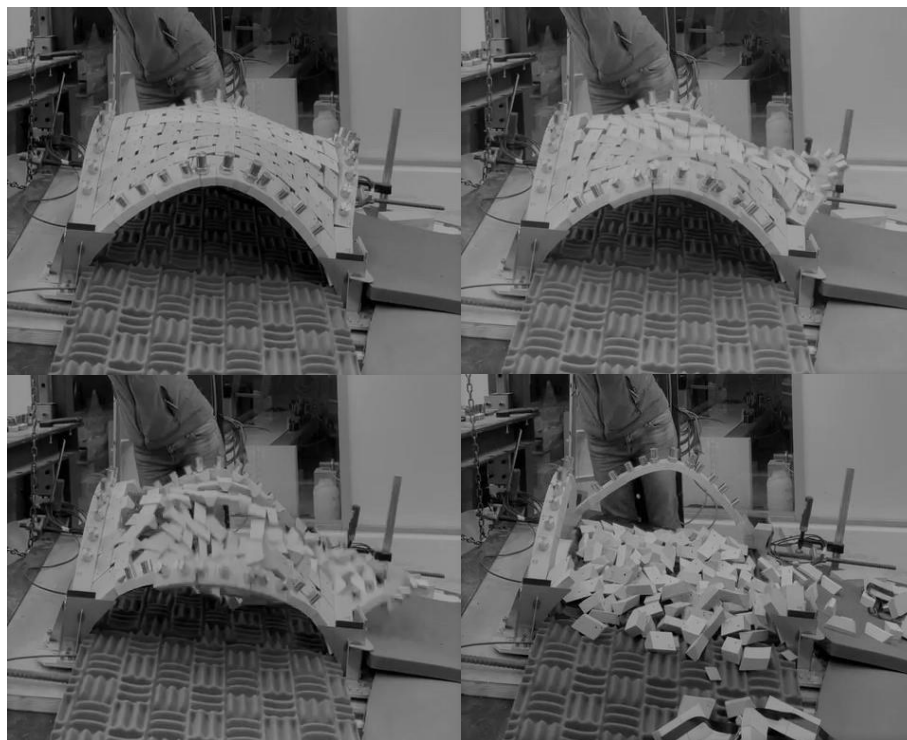
Figure 4-74. Damage results of the tilting tests with \Phi = 22.5^\circ : damage evolution in the lateral view ( p1-p3 ).
