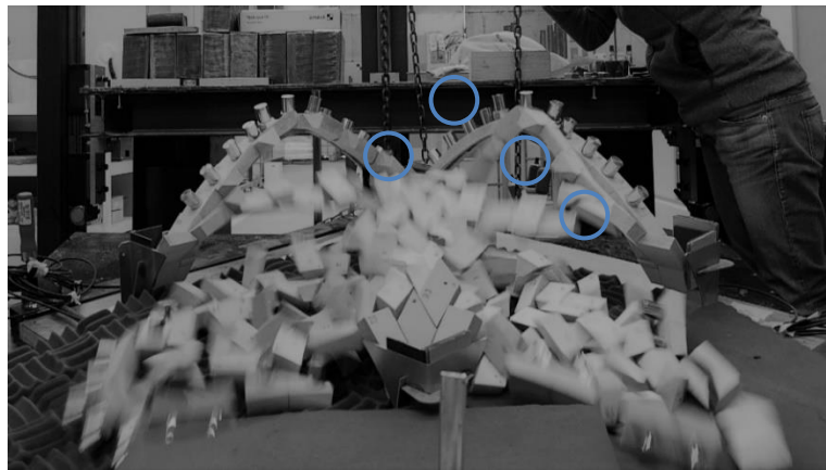
Figure 4-78 Damage results of the tilting tests with \Phi = 45^\circ (frontal view): detail of four hinge of the perimeteral vault row.
