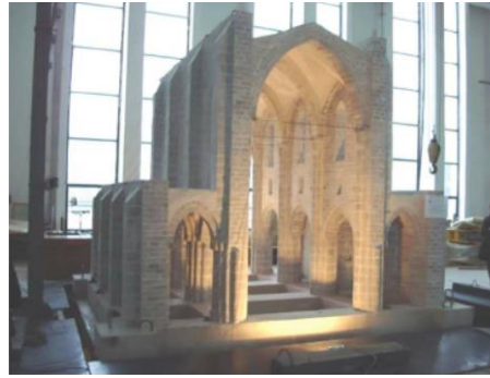
Figure 2-16. The 1:5.5 scale model and positioning on the shaking table (de Matteis & Mazzolani, 2010).
