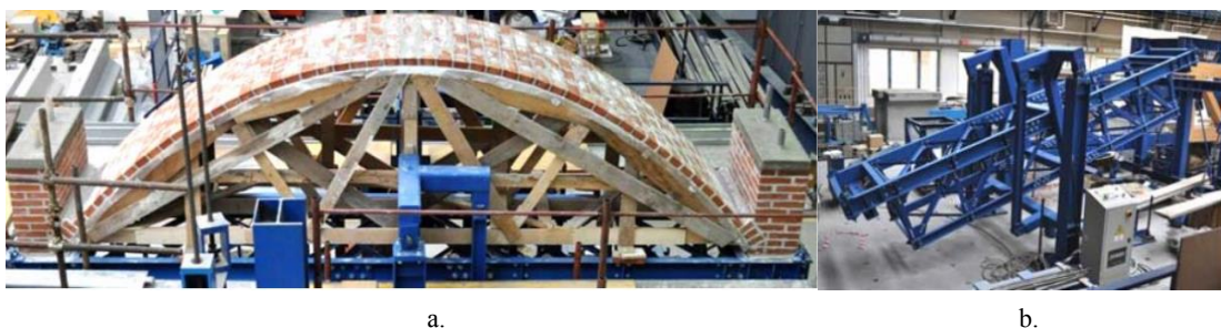
Figure 2-15. Test of the full-scale model of the single-leaf barrel vault: a. General view, b. Special testing bench (Ferrario et al., 2012).
