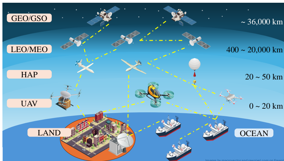
Figure 1.1: The envisioned integration of NTN, made by UASs, HAPs, and satellites, with land and ocean TNs for 6G communications. Altitudes reported on the right are indicative [11].
