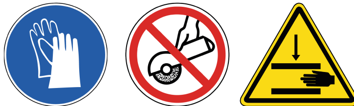
Figure 3: Examples of international safety symbols. From the left: a mandatory symbol, a prohibition symbol and a warning symbol (from UNI EN ISO 7010:2012 [36])
