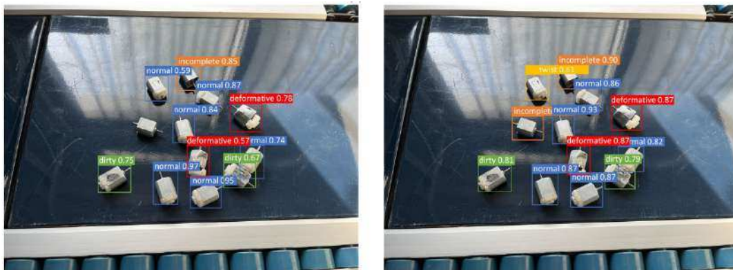
FIGURE 3.4: Surface imperfections Detection [15]
