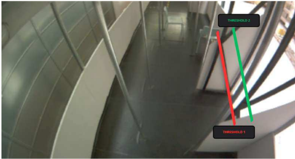
FIGURE 4.17: Inward and outward thresholds.
