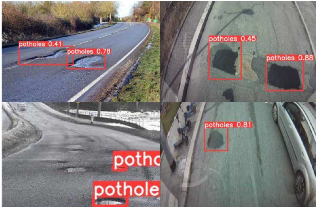
FIGURE 4.10: Potholes detection example.
