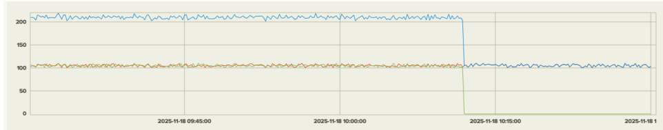
Figure 2.19: GPON power consumption with BNG consolidation [134].
